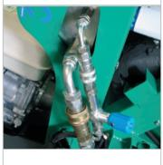
POWER TAKE-OFF WITH RAPID CONNECTION It allows the easy installation of a hammer (version 08).
